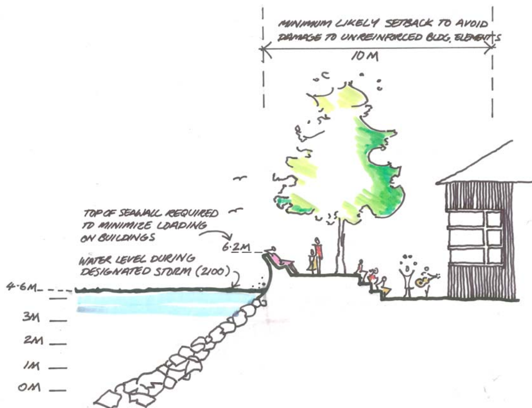
Figure Six – Cross Section of the Northwestern Corner of the Granville Island with Extended Protective Seawall, 2100
